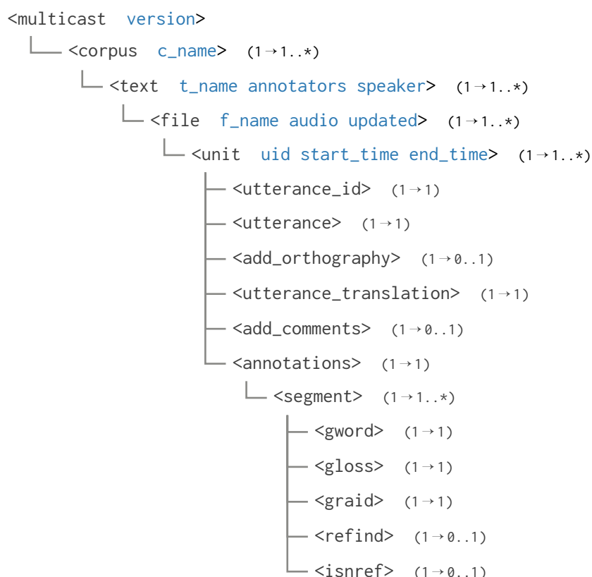
Figure 3 The structure of the Multi-CAST XML files. Attributes are given in blue. Cardinalities: (0..1) ‘zero or one’, (1) ‘exactly one’, (1..*) ‘one or more’.
